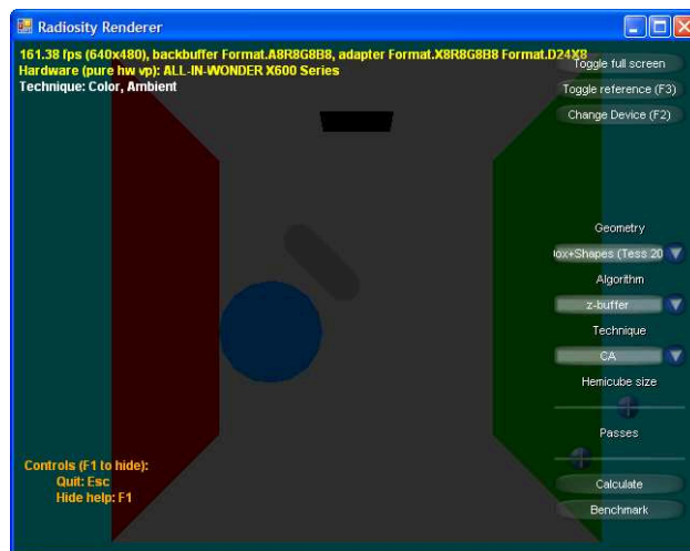
Fig. C.2: A simple scene, rendered using technique CA. Ambient color has obscured the entire image constantly. This technique runs in real time at more than 30 frames per second.
