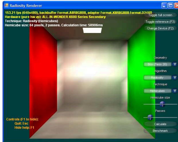
Fig. C.9: An empty box, similar to the Cornell box, rendered using the radiosity method described in this work. This scene took 58 seconds to calculate, but is presented in real time at more than 30 frames per second.
