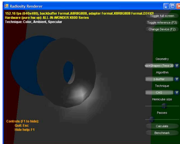
Fig. C.4: Detail of specular lighting, rendered using technique CAS. Note how per-vertex lighting forms artifacts in the floor. This technique runs in real time at more than 30 frames per second.
