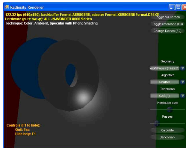
Fig. C.6: Detail of specular lighting, rendered using technique CAS(P). Per-pixel lighting has solved all artifacts, and lighting is now smooth. This technique runs in real time at more than 30 frames per second.
